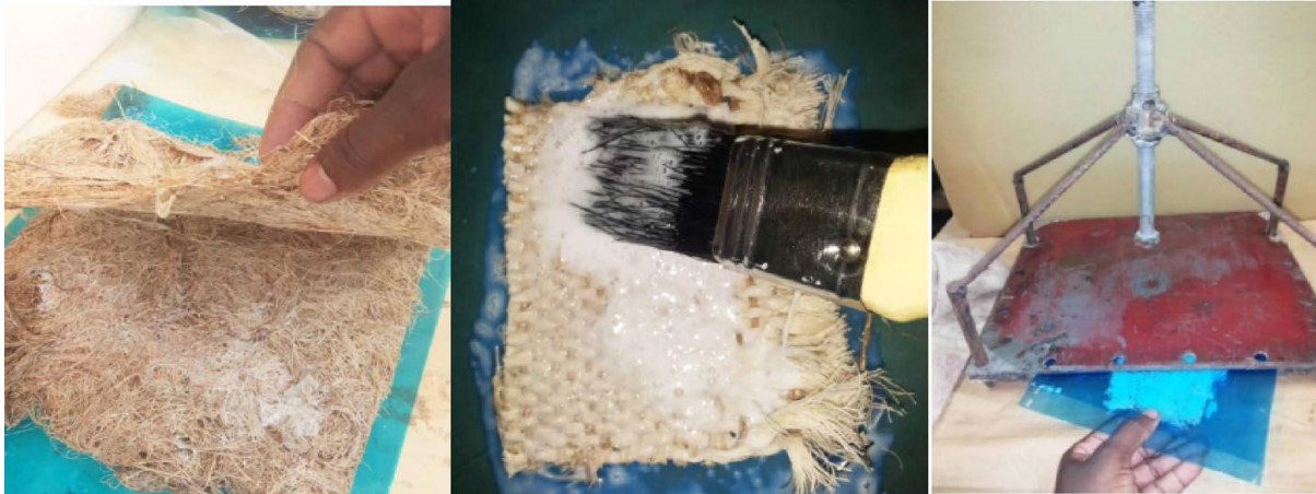
Figure 3: PVA application and compression process.
