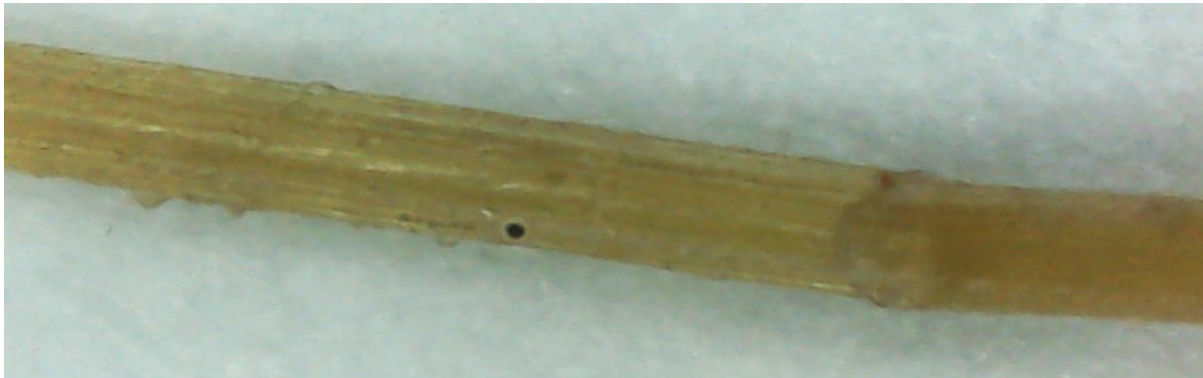
Figure 6: Digital optical microscopic view single (200 \times ); showing nod along the fibre axis.
