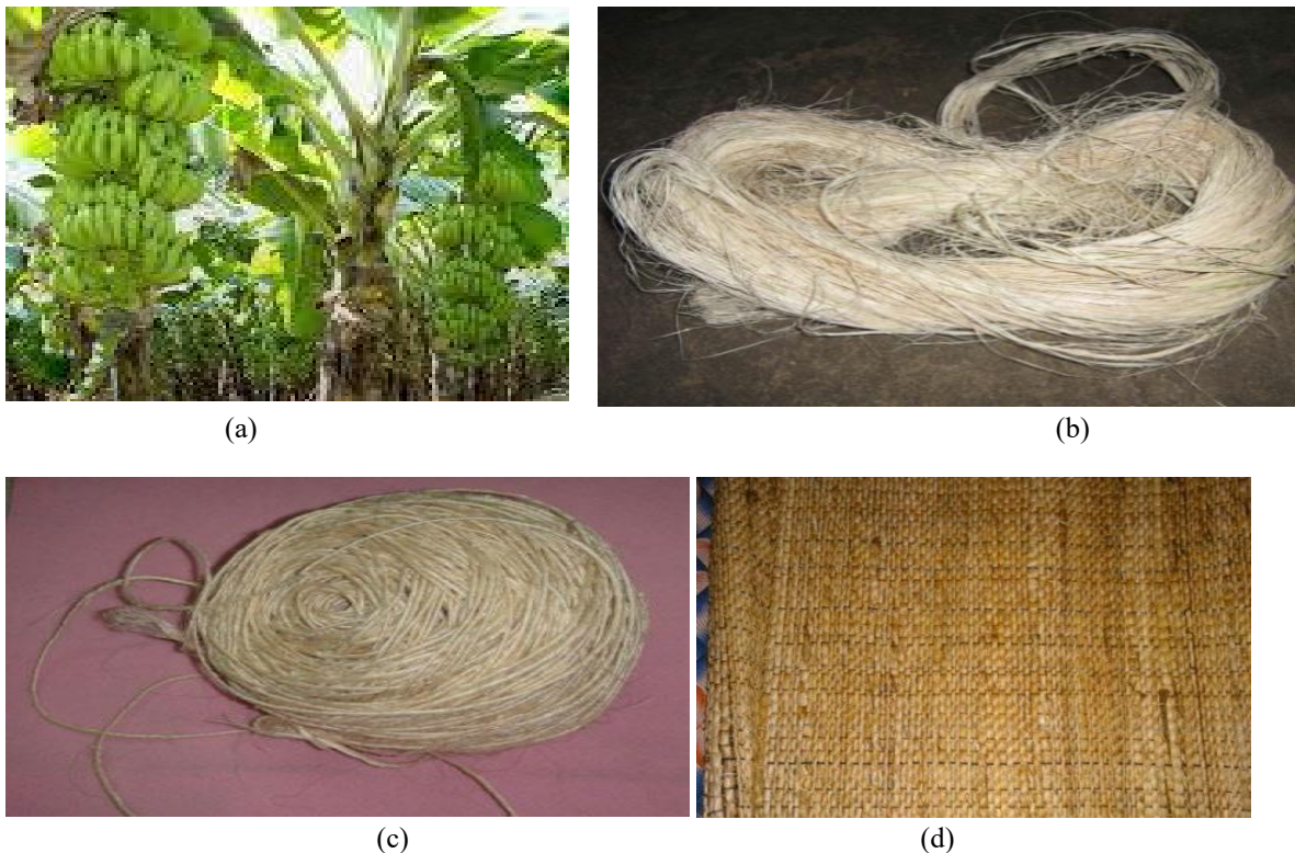
Figure 1(a – d): Preparation of banana fiber rope mat; (a) banana tree, (b) extracted fiber, (c) prepared fiber rope, and (d) woven fiber rope mat
