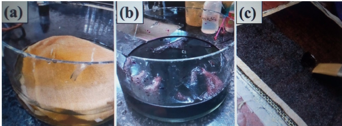
Figure 2: Chemical treatments: (a) 5 % NaOH, (b) 0.5 % KMnO 4 . (c) Hand lay-up method.
